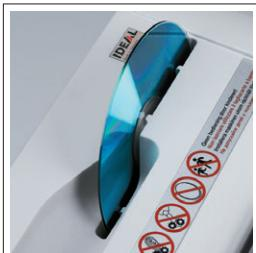
Separate feeding slot for the disposal of CDs and DVDs with a second cutting head. Photo cell for automatic start and stop.
